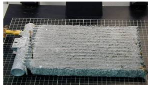
Microchannel coil 7000 hour Test
